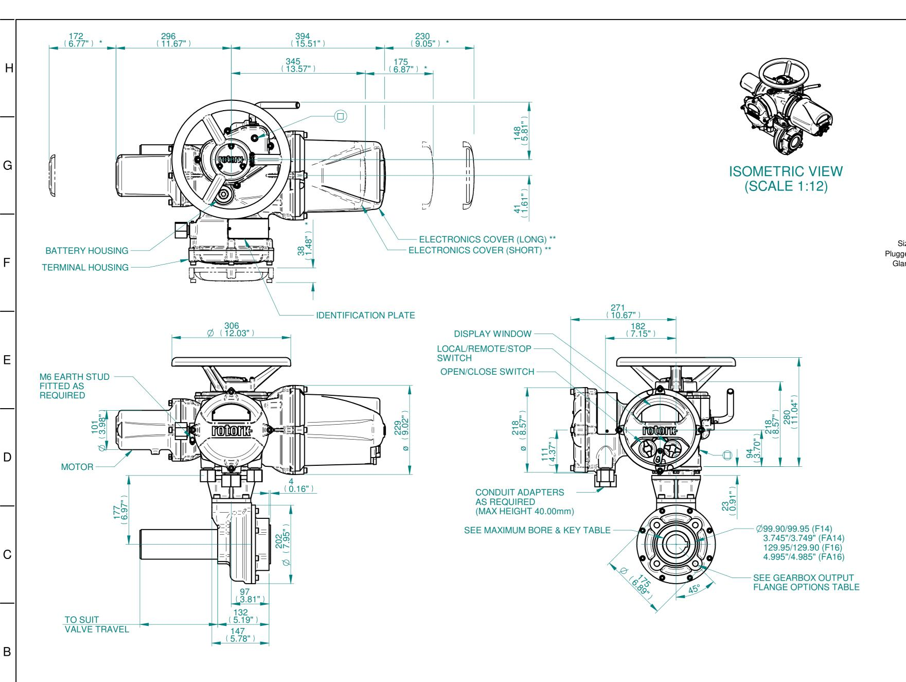
NOTES: :DIMENSIONS WITH '\*' INDICATE COVER REMOVAL ALLOWANCE :ELECTRONICS COVER OPTION "\*\*" WILL VARY DEPENDING ON CONFIGURATION :NETT WEIGHT = F14:51 kg/112 lbs, F16:53 kg/117 lbs:  $\bigcirc$  = OIL FILLER/DRAIN PLUG
