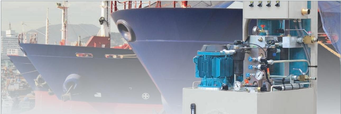
Our Hydraulic Power Unit features a stand-alone design: it can be hard-wired to the automation system or have an optional serial connection but in both cases the automation cannot stop or re-start it from remote: it may only read the information.
