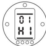
With [HI] displayed, an increasing set point signal will correspond to valve opening.
