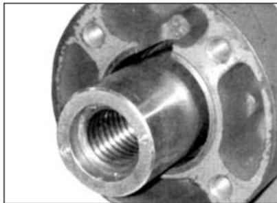
*Fig. 4.11 Type Z3 Drive Bush in Position 3*
