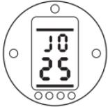
*Timer Set to Stop Pulsing when Opening Valve Reaches 25% Open*
