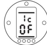
To enable remote diagnostics use the **+** or **-** key. The display will change to **[On]**.
