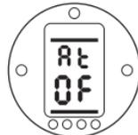
*Torque Switch Bypass Off*
