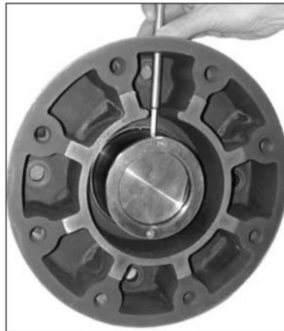
*Fig. 4.12 Tightening Retainer Set Screw*
