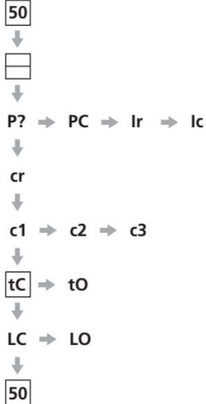
Using the + and – keys display recommended value. In the absence of a recommended torque value, try a low setting and increase until satisfactory valve operation is achieved.
