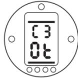
**[Ot]** in the Setting Field Indicates Open on Torque - default setting.
