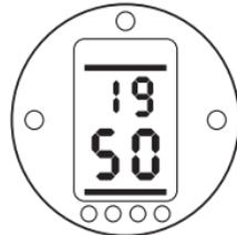
Example shows 19% (of rated) torque at 50% open position. Display torque range: [00] to [99]% of rated torque in 1% increments. For values of torque above 99% the display will indicate [HI].
