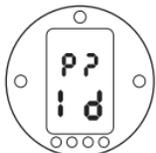
*The Actuator Function Settings can be protected by the Use of a Password*
