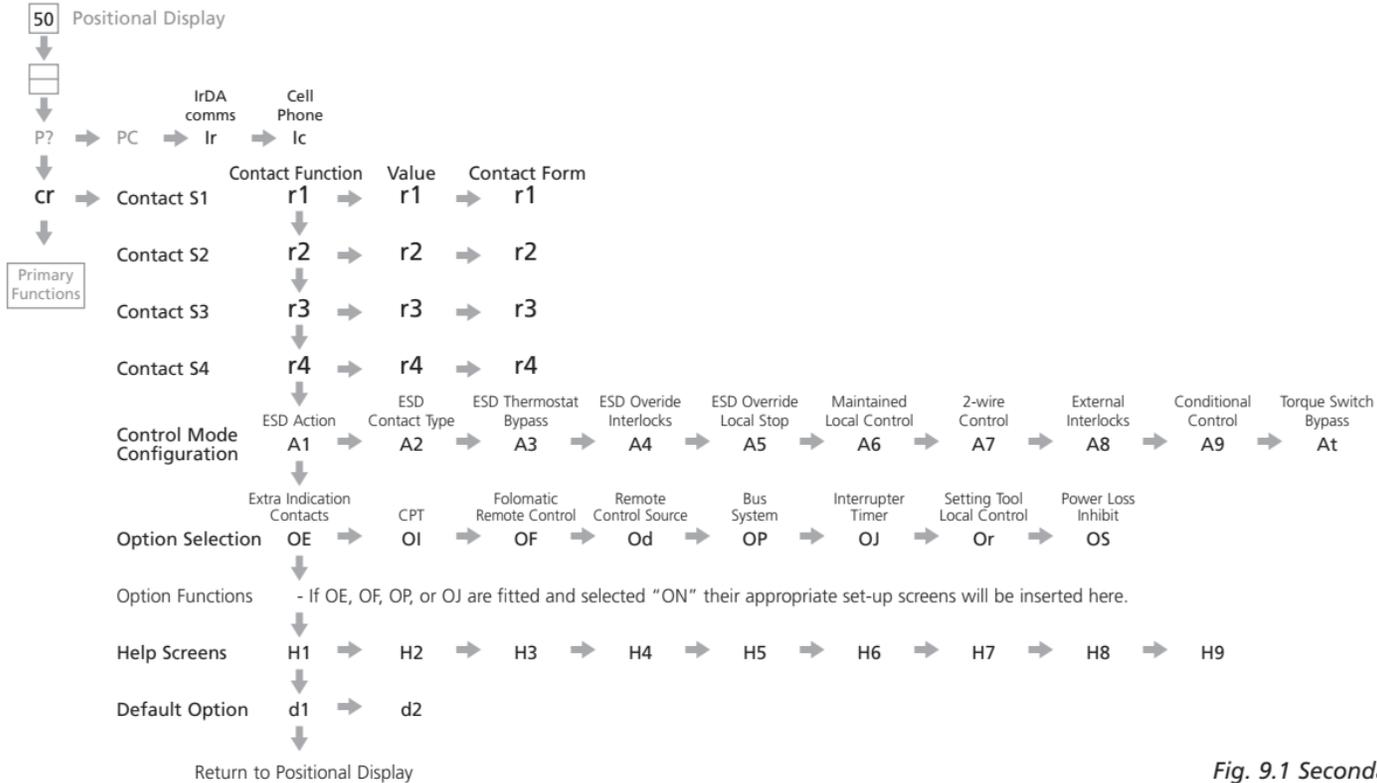
Fig. 9.1 Secondary Functions
