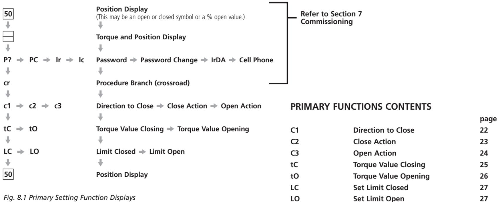
Fig. 8.1 Primary Setting Function Displays
