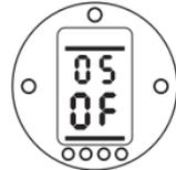
The protection may be enabled by using the + or – key to select [ON].
