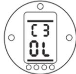
**[OL]** in the Setting Field Indicates Open on Limit
