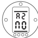
*Actuator Responds to a Remote, Normally Open ESD Contact Making (Signal Applied)*
