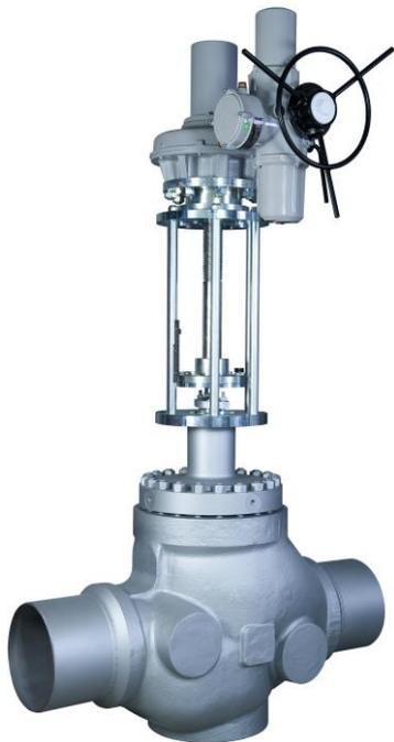
*A 20inch globe control valve fitted with a Rotork IQM actuator and IB bevel gearbox for installation on salt storage pipework in a solar power plant. (Photo: Flowserve Corporation)*
