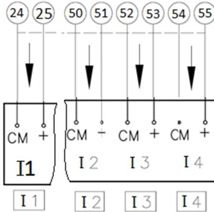
If additional remote inputs or outputs are required, the DIO option can be fitted inside the Centronik module. Each input can accommodate 20-60VDC, 60-120VAC. Current draw from each control input is 5mA at 24VDC, 12mA at 120VAC. Field wiring should have a maximum core to core capacitance of 2µF. For details of additional input settings please refer to PUB111-005.
