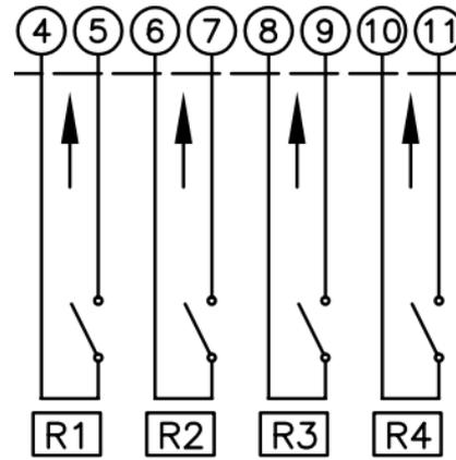
\* Monitor relay can be configured for faults only and will ignore the local control status.
