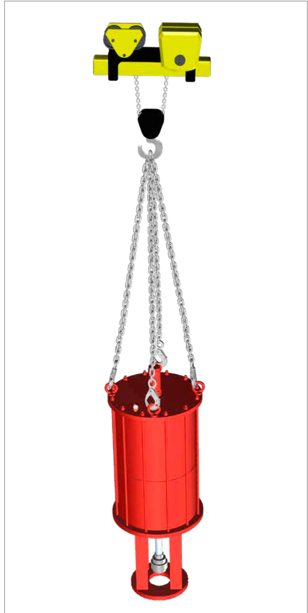
Fig 7.2 Lifting LPIS type 1 and type 2
