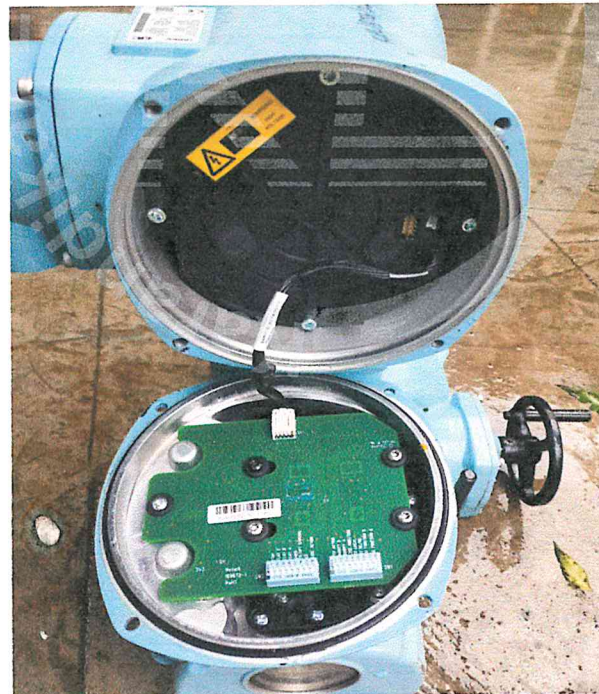
Pictute2: No ingress of powder & water observed
