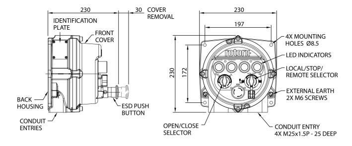
Dimensions in millimetres (mm).
