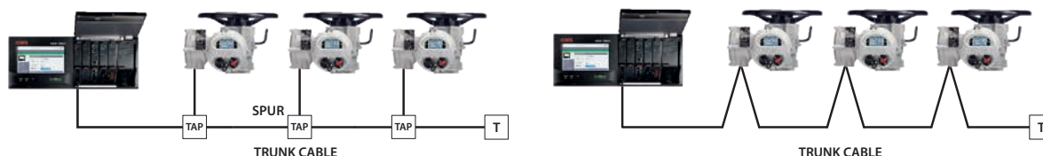
Fig 8.1.1: RS-485 Data Highway Topology – Single Channel
