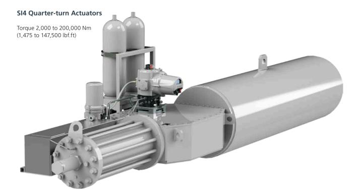
**SI4 actuators** offer the flexibility of customisation to suit specific applications and process conditions. They consist of a self-contained electro-hydraulic control module with a spring-return scotch yoke drive. This eliminates the high installation and maintenance costs associated with conventional electro-hydraulic systems which utilise central hydraulic power units.
