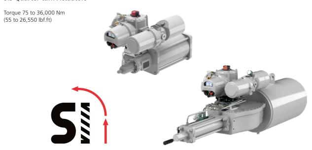
**SI3** actuators are compact and robust spring-return actuators designed for all types of ball, butterfly, plug valves and dampers. They consist of a self-contained electrohydraulic control module with a spring-return scotch yoke or rack and pinion drive. The actuators are available as either fail-safe clockwise or anti-clockwise. They can also be configured to stayput on loss of power supply.
