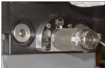
Fig. 6.1.1. Manual Override Handle
