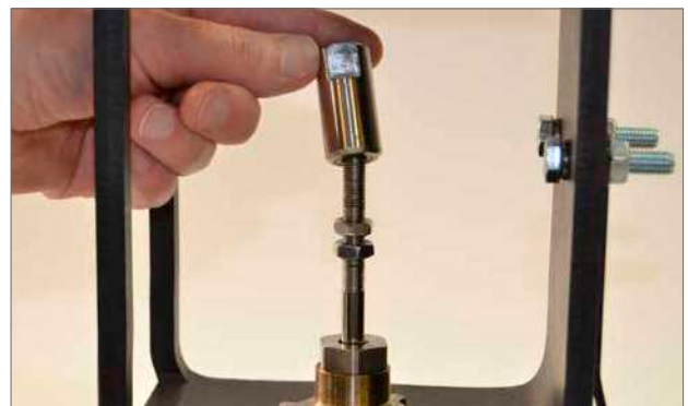
Fig 5.4 Coupling attachment to valve shaft
