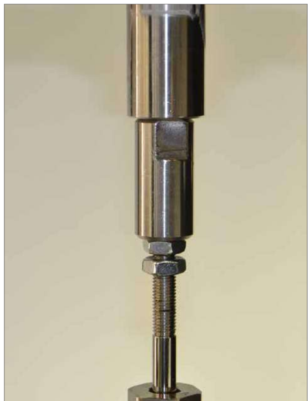
Fig 5.7 Connection of valve shaft and actuator shaft
