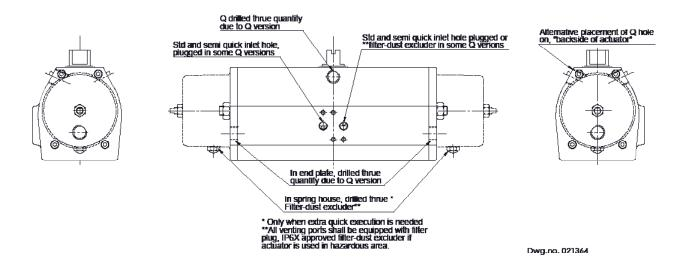
Dimension, thread type and number of hole for medium connection can be found on the RC...-...Q actuator sticker.
