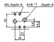
Hole pattern for solenoid valves acc, to EN 15714-3
