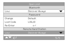
7.2 Navigate to SETTINGS > SECURITY and under the Remote Hand Station section, choose the level of Bluetooth access required for the RHS.
