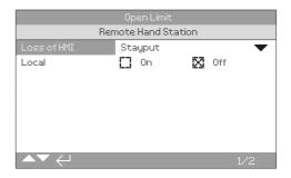
**Setting the Local mode** - The Remote Hand Station is intended to work when the actuator is set to Remote Control only, however you can configure the RHS to work when the actuator is set to Local Control. In this case both the RHS and actuator will allow local control, with the last issued command taking preference.
