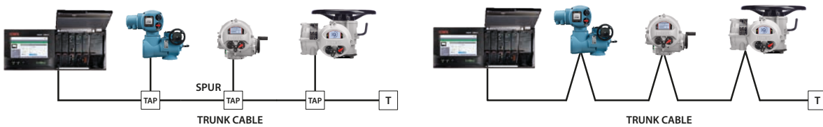
Fig 8.1.1: RS-485 Data Highway Topology – Single Channel
