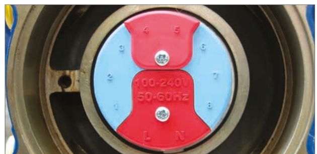
Fig 7.16 IS terminal block
