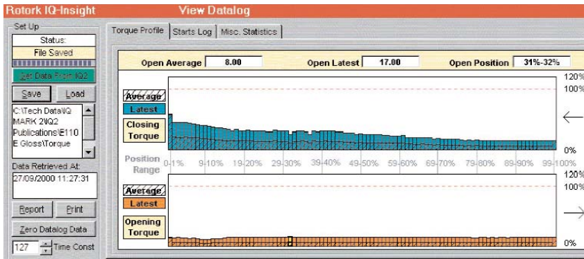
Sample of IQ-Insight downloaded data logger diagnostic information as displayed on a PC, showing the last recorded valve operating torque graph.
