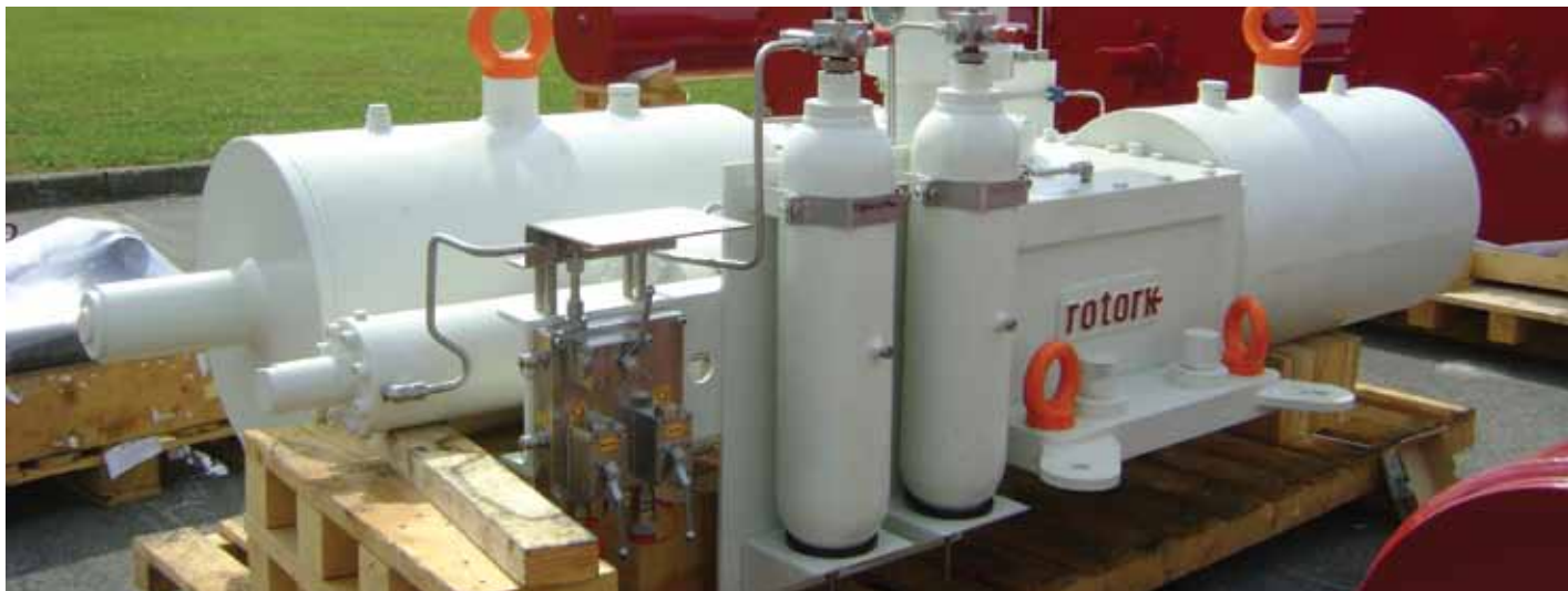
Fig 1 This spring-return rack and pinion actuator, model number GSR-2-490-110F/CX, will operate a 16 inch ANSI Class 900 ball valve installed on the eleven kilometre export pipeline from the Seth Platform off the coast of Egypt. This pipeline connects to the Tuna Platform export pipeline end manifold for onward transport to the shore via the TNW2 Platform. The actuator will operate an SSIV installed at a depth of 84 metres near to the Seth Platform, which, together with a check valve installed upstream of the ball valve, will prevent any gas backflow in the event of a pipeline or riser rupture in the proximity of the platform. The installation is very similar to the Rotork actuated SSIV package shown in Fig 2 that was previously supplied for the 24 inch export pipeline from the Tuna Platform. Both installations are equipped for pipeline pigging operations and fitted with superstructures for protection against accidental impacts and to prevent any interference with fishing activities.
