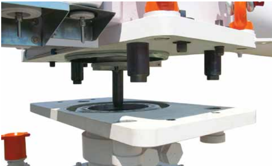
Fig 4 With the actuator removed in a simple lifting operation, the valve can still be operated by means of the ROV override on the spool piece (shown bottom left).
