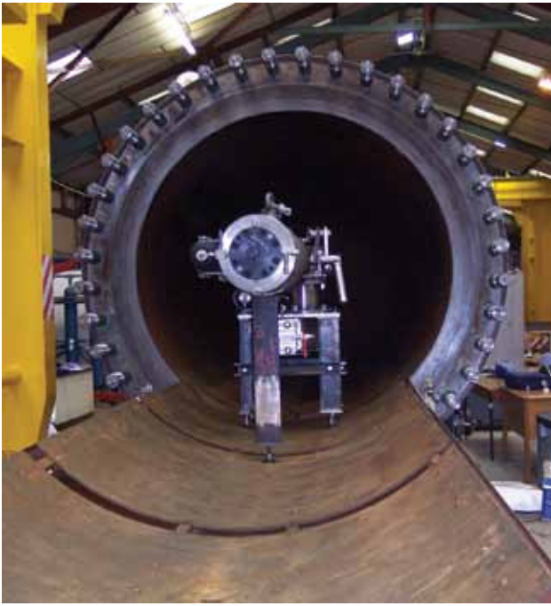
Fig 3 A hydraulic actuator undergoing preparation for pressure testing in a hyperbaric chamber at the Rotork Fluid Systems factory
