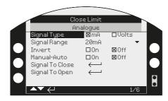
When analogue control is selected independent deadband and hysteresis adjustments are provided in the menu to optimise the control to suit the process conditions. The position against
