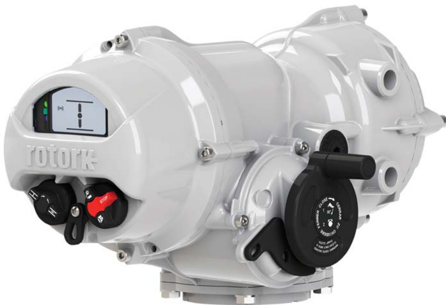
Fig 1 – IQT actuators are suitable for three phase, single phase or DC power supplies, with a torque output range of up to 2,000 Nm available for isolating, regulating and modulating duties. The motor always runs in the correct direction, irrespective of supply type and connection. In addition, the output speed can be non-intrusively adjusted over a 4:1 range without affecting the output torque. All valve interface bases conform to ISO5211 or MSS SP 101 and are fitted with removable couplings.
