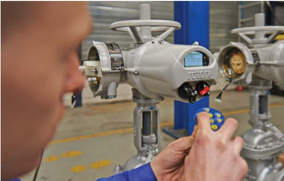
Fig 2: In recent years the development of intelligent actuators with diagnostic capabilities has greatly increased the ability to seamlessly include actuators in the asset management plan and plant operations.
