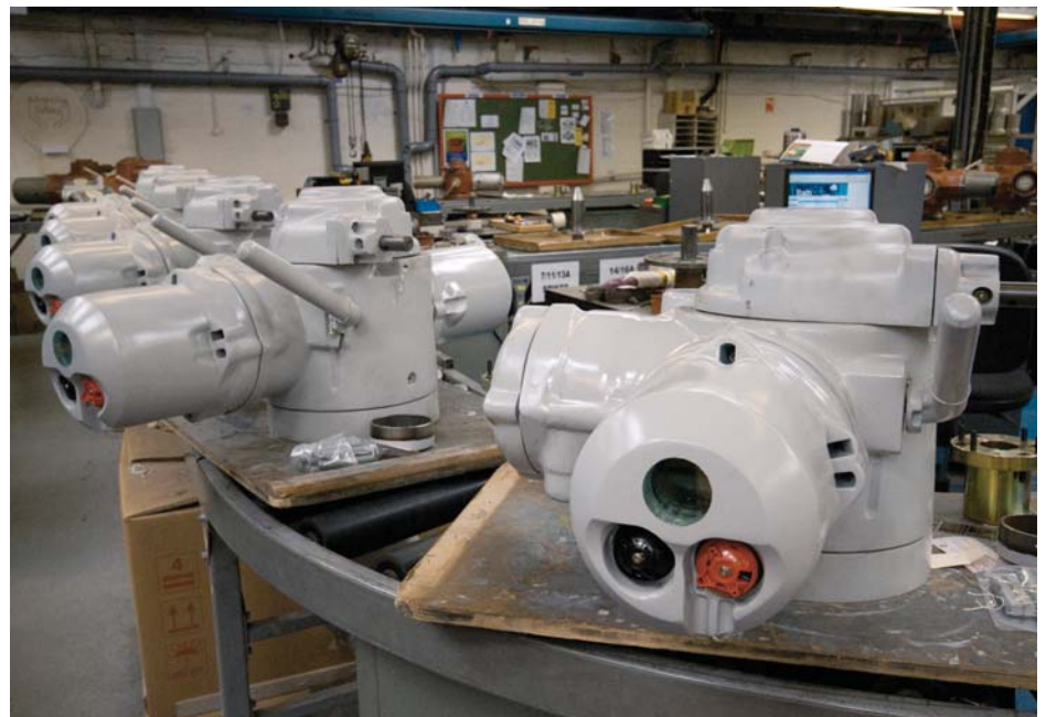
Fig 2: Rotork IQ actuators with System-E intumescent fireproof coatings, en-route to the Tupras Izmit Refinery.
