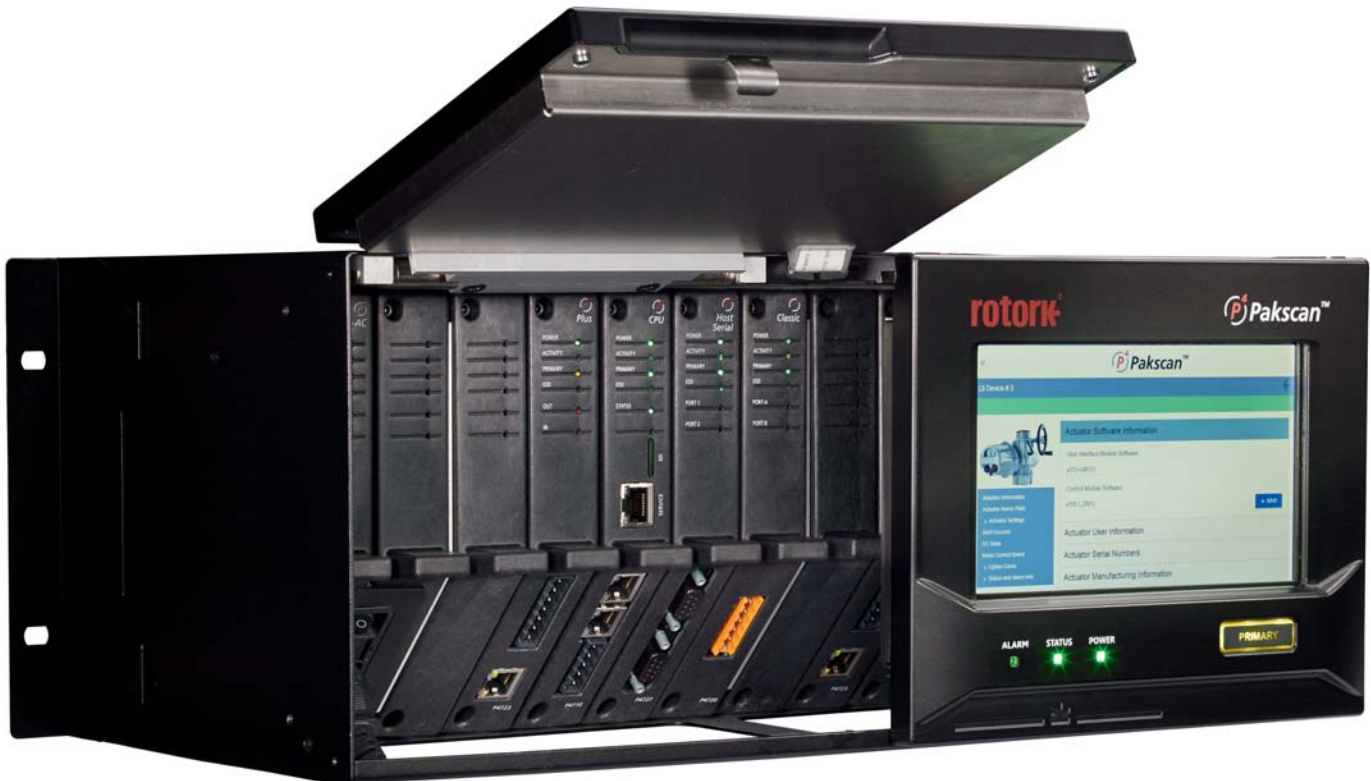
Each Pakscan network, wired or wireless, is supervised by the Pakscan Master Station, which links the plant network with the control system. Pictured here, the latest Pakscan P4 Master Station has introduced an ultra-fast Plus network.
